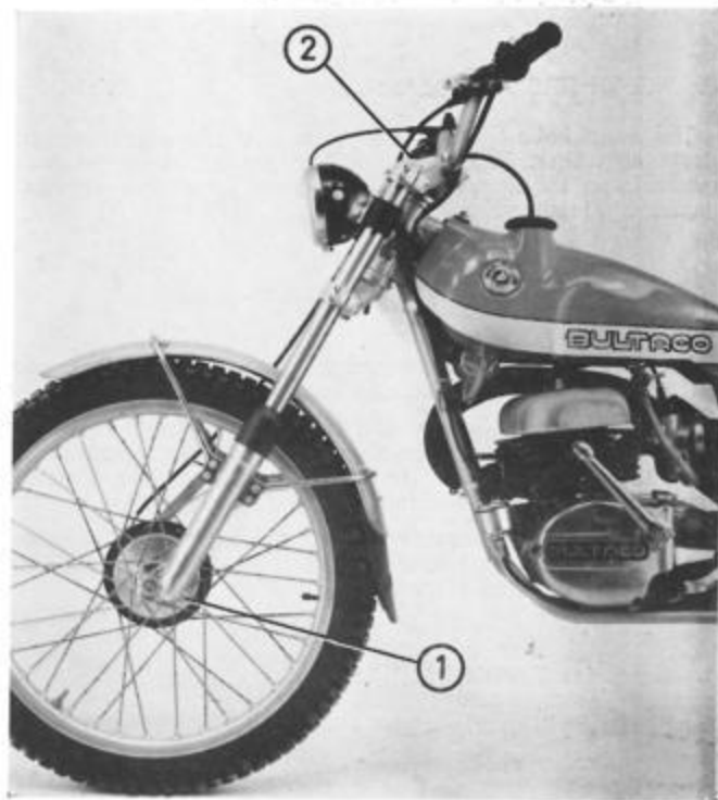
1. The drain screw. — 2. The filler plug.
